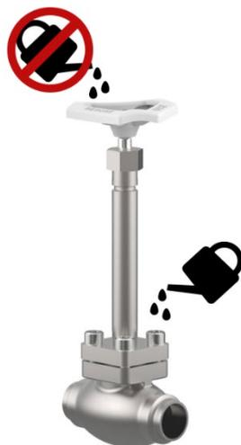
To speed up the thawing of the filling valves, the housing can also be sprayed with water. The stuffing box packing must be protected from water.
